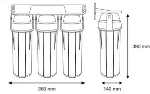
Dimensions (H x W x L): 390 x 140 x 360 (mm) Connection adapter: 1/2" Working Temp.: 2°C - 45°C (35°F - 113°F) Working Pressure: 6 bar (90 PSI)
